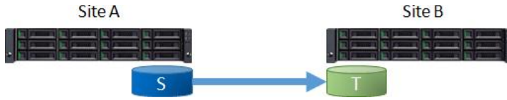
Figure 4-12 One-Directional Remote Replication
